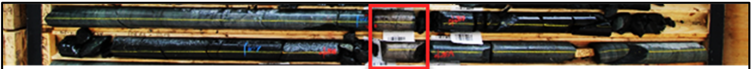
Figure 5. Two distinct massive sulphide intercepts in drill hole DS-21-005.
